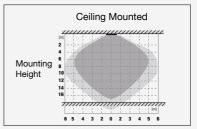
MEGAMAN® KEO 2 microwave sensor detects movement within around 5-6m radius horizontally and / or 10-12m vertically beneath sensor, and only lights up when movement detected for energy saving.
