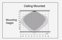
MEGAMAN® KEO 2 microwave sensor detects movement within around 5-6m radius horizontally and / or 10-12m vertically beneath sensor, and only lights up when movement detected for energy saving.
